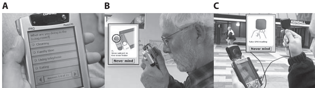
Figure 6. (A) Context-aware ecological momentary assessment protocols are being tested on personal digital assistants running custom MIT software that offers a variety of options for acquiring self-report data from users or subjects in experiments. This image shows one screen from a sampling protocol used in a study to collect training data for algorithms that automatically detect activities in the home setting. (B) The software permits the use of data collection sensors, such as cameras, microphones, and a wireless heart rate monitor. This image shows a user taking a picture with the camera plug-in and one of the built-in tutorial screens. (C) The software can also either prompt for sensor data, such as taking a global positioning system (GPS) reading, or use continuously acquired sensor data to trigger a set of self-report questions to be presented. Here, a user is acquiring a GPS sample, which is done by holding up a small antenna plugged into the GPS device. These technologies are bulky, but in less than 10 years, the enabling technology (e.g., GPS) will be standard in mobile phones. From "Technological Innovations Enabling Automatic, Context-Sensitive Ecological Momentary Assessment," by S. S. Intille, 2007. In A. Stone, S. Shiffman, A. Atienza, and L. Nebeling (Eds.), The Science of Real-Time Data Capture: Self-Reports in Health Research , pp. 308–337. Oxford: Oxford University Press. Copyright 2007 by Oxford University Press. Reprinted with permission.
