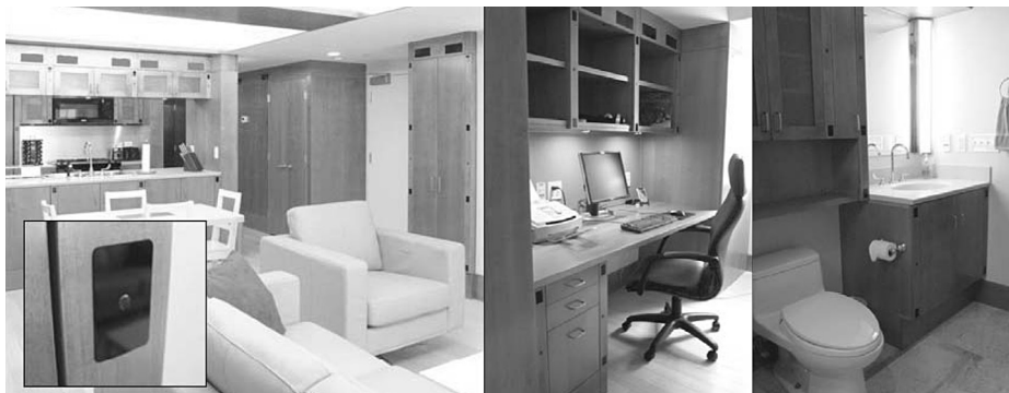
Figure 3. The PlaceLab living room and kitchen, office, and master bath. All of the observational sensing is built directly into the cabinetry. Although the sensors are ubiquitous, they become part of the design aesthetic (small black windows). The inset in the left image shows a microphone. From "A Living Laboratory for the Design and Evaluation of Ubiquitous Computing Technologies," by S. S. Intille, K. Larson, J. S. Beaudin, J. Nawyn, E. M. Tapia, and P. Kaushik, 2005. In CHI '05: Extended Abstracts on Human Factors in Computing Systems . New York: ACM Press. Copyright 2005 by ACM. Reprinted with permission.
